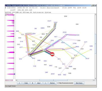
Figure 17: A routing status following that of Fig. 16 where shorter AS-paths disappeared due to the propagation of the withdrawal.
