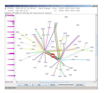
Figure 16: A BGP beacon periodically announcing and withdrawing the prefix 198.133.206.0/24 from 2005-05-10 13:10:00 UTC to 2005-05-11 13:10:00 UTC. Note the regular patterns of activity in the time panel which correspond to the beacon being announced and withdrawn with a period of exactly two hours. The picture shows the routing status just before a withdrawal.
