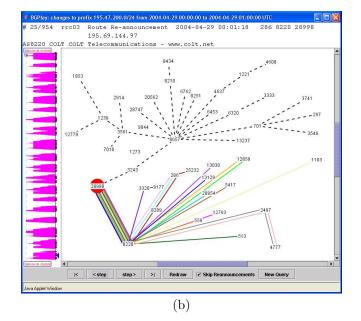
Figure 11: A prefix in AS28998 periodically oscillating between two routing states: (a) all collector peers see the prefix through one of its ISPs, AS3243; (b) some peers change their paths to the prefix so that they go through another of AS28998's ISPs, AS8220. The time panel shows bursts of BGP activity occurring approximately every three to four minutes. Examination of the routing graph suggests that these may be caused by a connectivity problem between AS28998 and AS8220.
