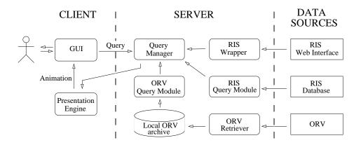
Figure 2: The system architecture.
