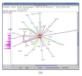
Figure 15: The new prefix 84.128.0.0/11 is announced at about 2004-03-16 08:08:00 UTC: (a) before the announcement; (b) after convergence. Studying the order of routing events can provide insight into the way in which timing factors influence the propagation of announcements and can lead to path changes during convergence.
