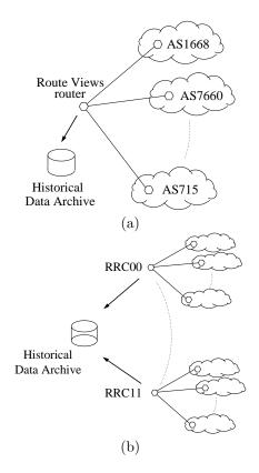
Figure 1: The architecture of ORV (a) and of RIS (b).
