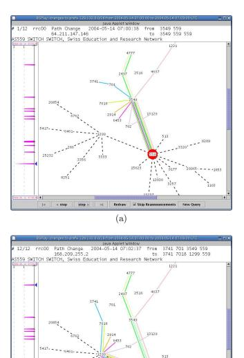
Figure 14: Studying the effects of traffic engineering. AS559 (SWITCH) changes the AS prepending on the routes it announces to one of its upstreams to influence other ASes's routing toward itself: (a) before the change; (b) after the change. Note that a number of collector peers have switched paths and now use AS1299 instead of AS3549 to reach AS559. Using BGPlay the operators of AS559 were able to see in near real-time whether the configuration change had had the desired effect.
