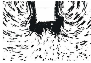
FIG. 1.6. Visualization of 1\mu\text{m} -sized particle trajectories near a spike in the cathode in an ECD in a vertical cell (cathode above anode) giving rise to a locally unstable flow. To show the motion of tracer particles, 200 digital images were superimposed: from 40 to 60s. Copper sulfate solution concentration is 0.1\text{M} with 30% glycerol in weight, the cell dimensions are 70 \times 10 \times 0.127\text{ mm}^3 , the applied constant current is 2\text{ mA} , and the spike dimensions are 1 \times 0.5 \times 0.127\text{ mm}^3 .
