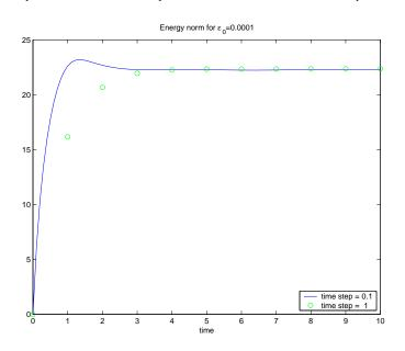
FIG. 4.2. Stability of the numerical method demonstrated by the behavior of the energy norm
