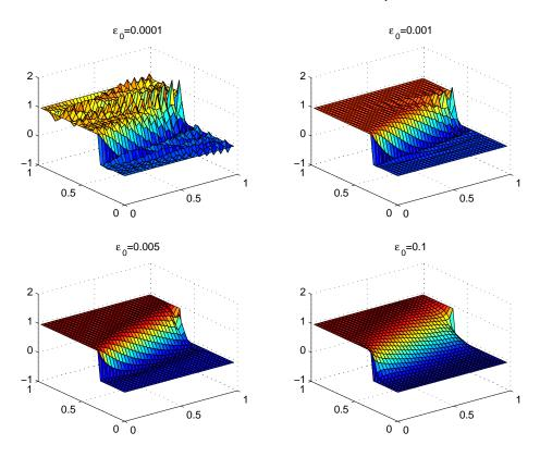
FIG. 4.1. Spatial stability of the steady-state solution for various choices of the artificial viscosity parameter  $\epsilon_0$ .
