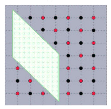
FIG. 4.3. The parallelogram blocking technique for the red-black Gauss-Seidel
