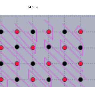
FIG. 4.4. The new layout of data in memory for Gauss-Seidel using the cache aware data layout scheme. Here too, the size of a cache-line is 4.
