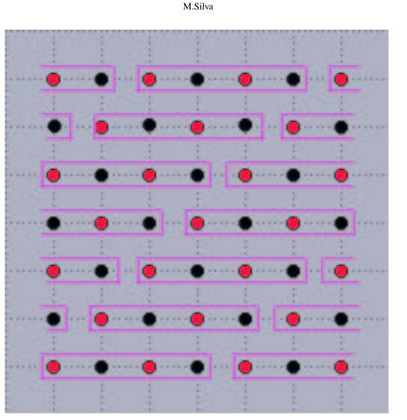
FIG. 4.2. Standard layout of the red-black Gauss-Seidel unknowns in memory for a cache-line size of 4.
