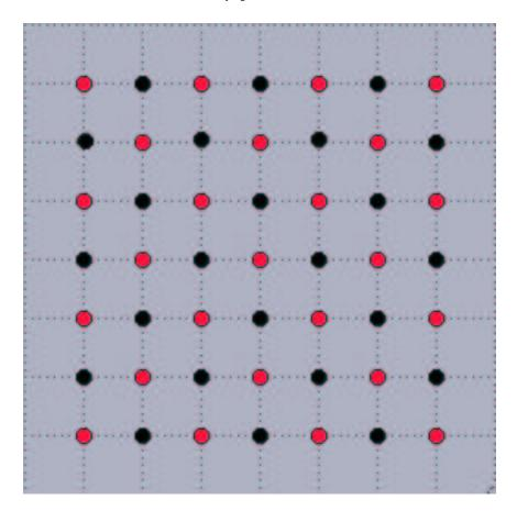
FIG. 4.1. Red-black ordering of the unknowns for the red-black Gauss-Seidel algorithm. Here, the size of the grid is 9 and we have not shown the boundary nodes.
