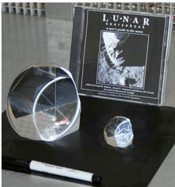
Figure 7: A 10 cm solid cube corner reflector was recently qualified for the lunar environment. Also shown for comparison is a 3.8 cm Apollo engineering model cube corner [11]. (Image credits: Douglas Currie.)
