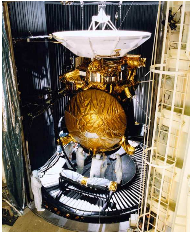
Figure 4: The Cassini spacecraft during pre-launch testing. Reference [68] gives a popular discussion of the Cassini mission, the spacecraft, and its instrumentation (photograph courtesy NASA/JPL-Caltech).
