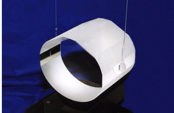
Figure 5: Prototype ‘monolithic’ fused silica test mass suspension. The mass (3 kg) here is of 12.5 cm diameter. Note final suspension will use four fibres.
